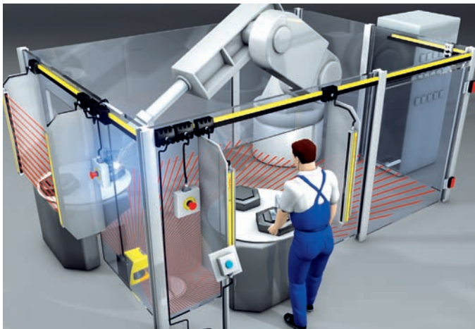
A typical robot application with 2 release circuits for switching off the dangerous movement
