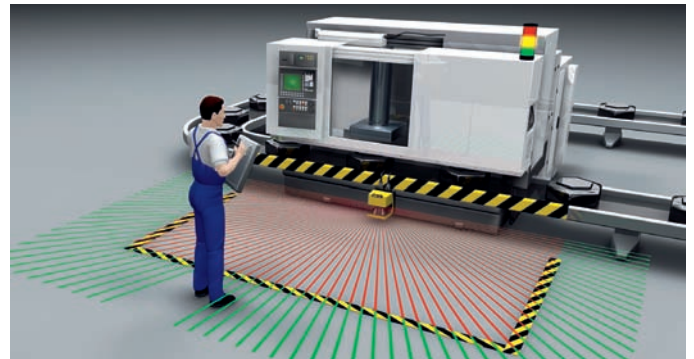
Danger area guarding at stationary machinery: Effective use of the detection zone/warning zone combination for people and machine safety
